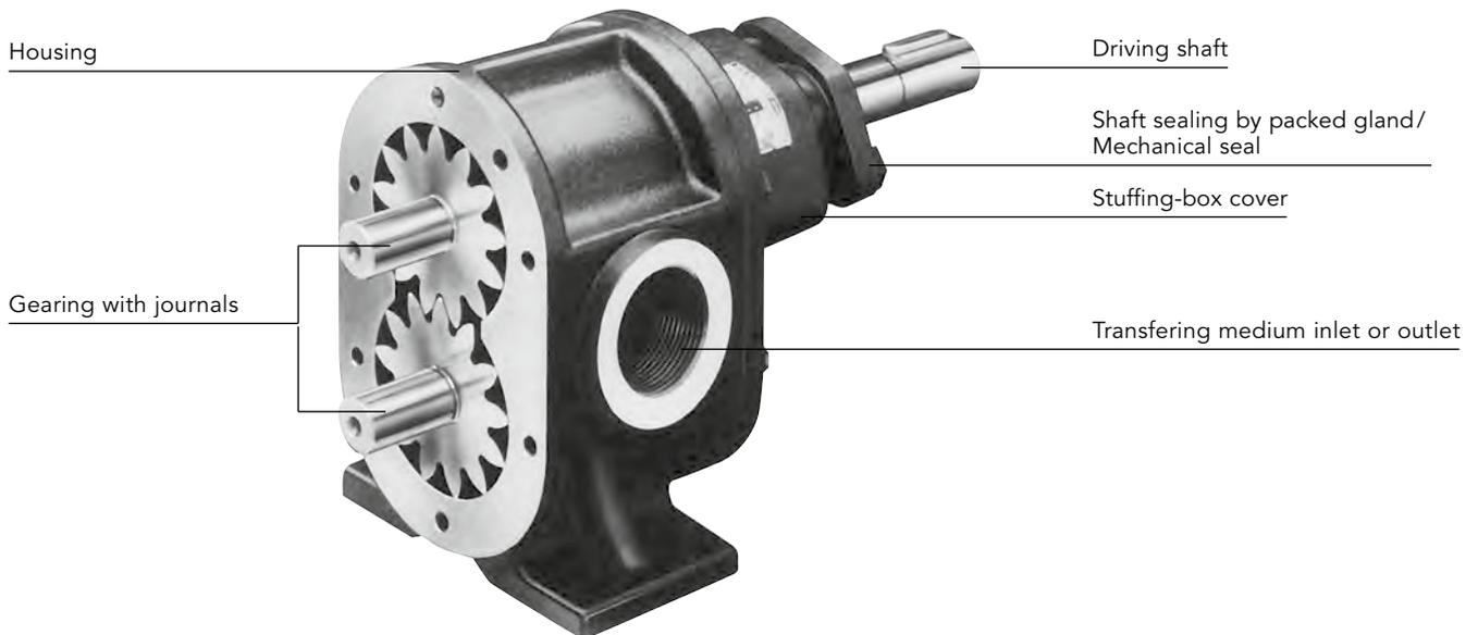
**Basic construction of BTH (rear bearing cover removed)**
